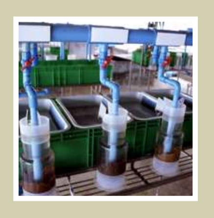
Tanks containing harvested fish eggs. When the eggs hatch, the tiny fish fry will swim to the surface and spill over into trays—an example of efficient, simple technology based on sound scientific know-how.
